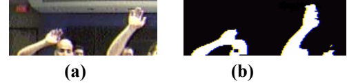
Figure 7. Skin detection results; (a) original image, (b) matching pixels in normalized RGB space.
