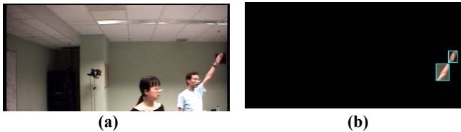
Figure 13. Test of distracter rejection: (a) the distracter (the student in the center of the image) has just appeared in the scene (b) detected targets.
