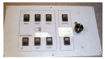
Figure 2. The HC-12 controlled physical button panel as an alternative to a graphical touch-screen interface. This panel provides manual override control of the room lights, projector, screen, drapes, and volume, without the need for distracting, hierarchical menus. Furthermore, the volume knob is context-sensitive, adjusting either the volume of the VCR when a tape is playing, otherwise, that of the instructor's microphone.
