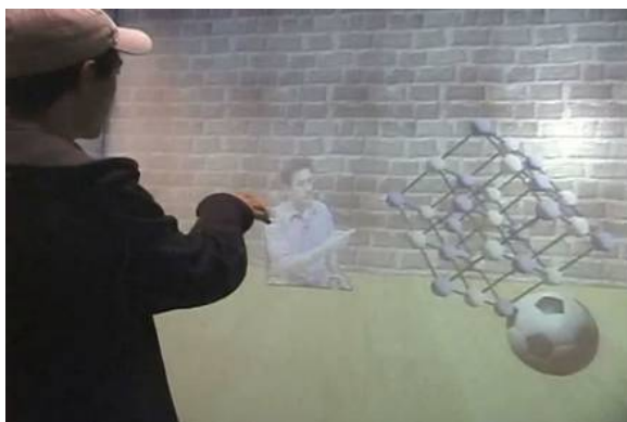
Figure 2: A projected remote participant, rendered as a “2D cardboard cutout” in the virtual museum space. The video display is transformed in real time based on the position of the viewer in order to provide a correct perspective view.
