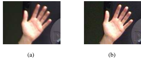
Figure 4. Motion blur reduction in a high-resolution frame. (a) Frame affected by motion blur (b) Frame after motion blur reduction.
