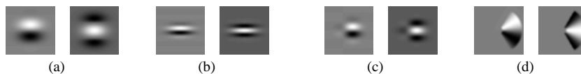
Figure 3: Quadrature pair of Gabor filters at frequency of 0.75 with (a) \sigma_x=\sigma_y and (b) \sigma_y = (\frac{1}{2})\sigma_x , (c) OneSided filters [12], and (d) Wedge filters [15]
