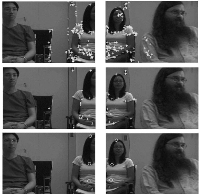
**Figure 2. Two neighboring input images are shown, with crosses indicating SIFT feature positions. In the first row, these are restricted to the human subject who appears in the overlapping region, whereas, in the second row, only the crosses from a nearest neighbor match are retained. The circles in the third row represent the RANSAC inliers, which are used to estimate initial camera motion model parameters.**
