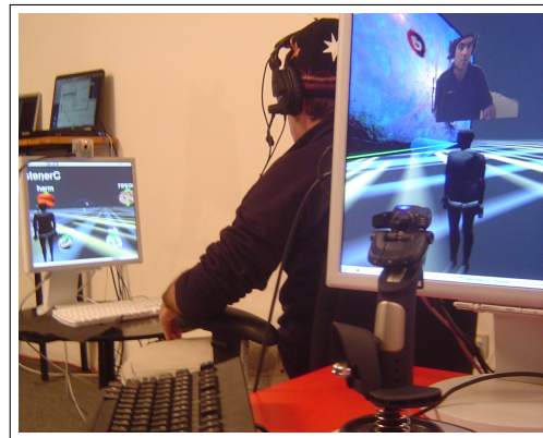
Figure 3: A prototypical deployment, where a remote user is seen as a virtual avatar with a video stream above his head. Though difficult to see in this figure, the avatar has a diffusion cone emanating from his head that indicates the direction of the emitting sound.
