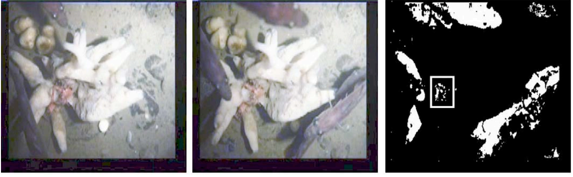
Fig. 1. Example of change mask generation. Sample frame from time t (left), sample frame from time t + 50 (middle), and change mask after thresholding the intensity difference between the two frames (right). Note that in this example, the significant objects are contained exclusively in the rectangular bounding box.
