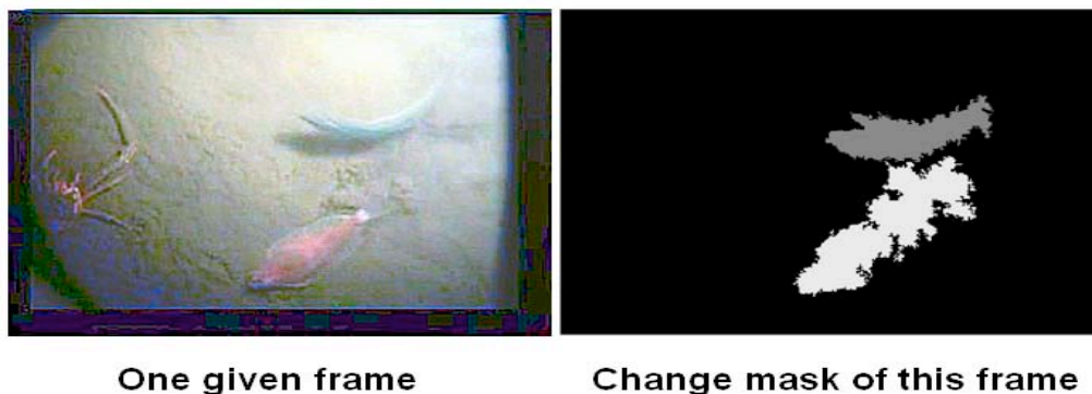
Fig. 6. A sample video frame (left) and the corresponding change mask (right). For the purposes of illustration, regions corresponding to significant objects (the lower fish) are shaded in a lighter color than the distracter.
