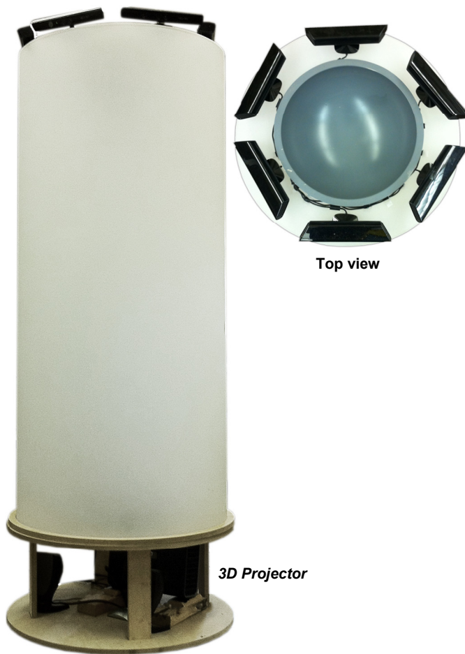
Figure 2. TeleHuman hardware: a cylindrical display surface with 6 Kinects and a 3D projector inside its base.
