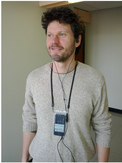
Fig. 1: Neck carrier holding the iPhone for hands-free use in an upside down orientation, facing outward, to provide easy access to the touchscreen. Device is in a plastic pouch that protects it from the elements, yet does not interfere with touch events. User is wearing Airdrive headphones that do not obstruct the ear canal, so is able to hear ambient noise, important for safety in a busy urban environment.
