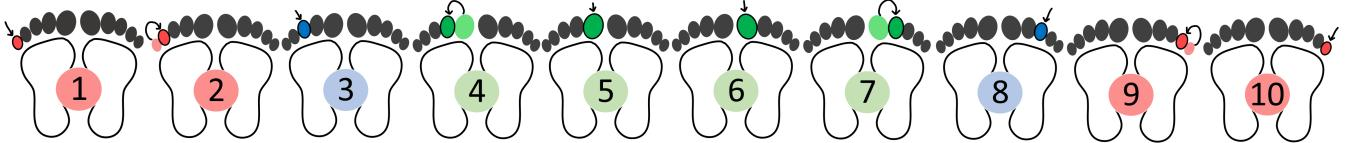
Fig. 2: Final design of HapToes for both feet. For numbers 1, 3, 5, 6, 8 and 10, a long vibration of 1200 ms is rendered on the targeted toe (darker color). For the remaining numbers 2, 4, 7 and 9, a short vibration of 400 ms is rendered on the closest edge toe, followed by a longer vibration of 800 ms on the targeted toes (darker color).
