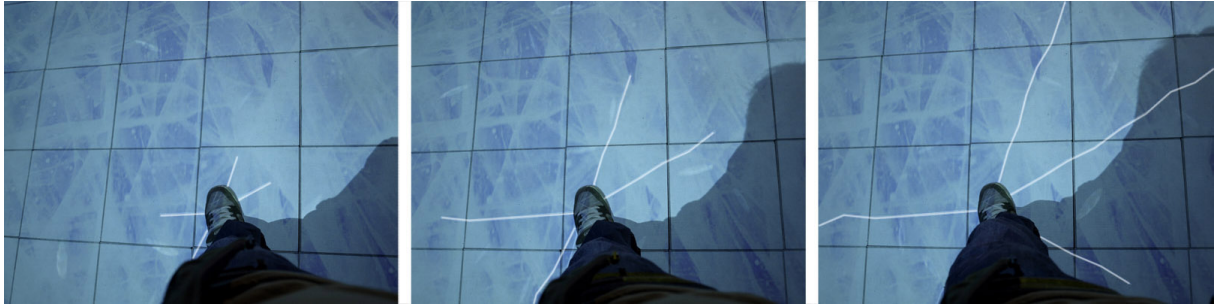
Figure 3.13 The crack arms propagate outwards from the foot. The lines have been enhanced in the photographs to show the effect.
