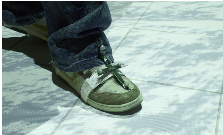
Figure 3.7 Vicon markers are attached to the user's feet using an elastic Velcro strap.
