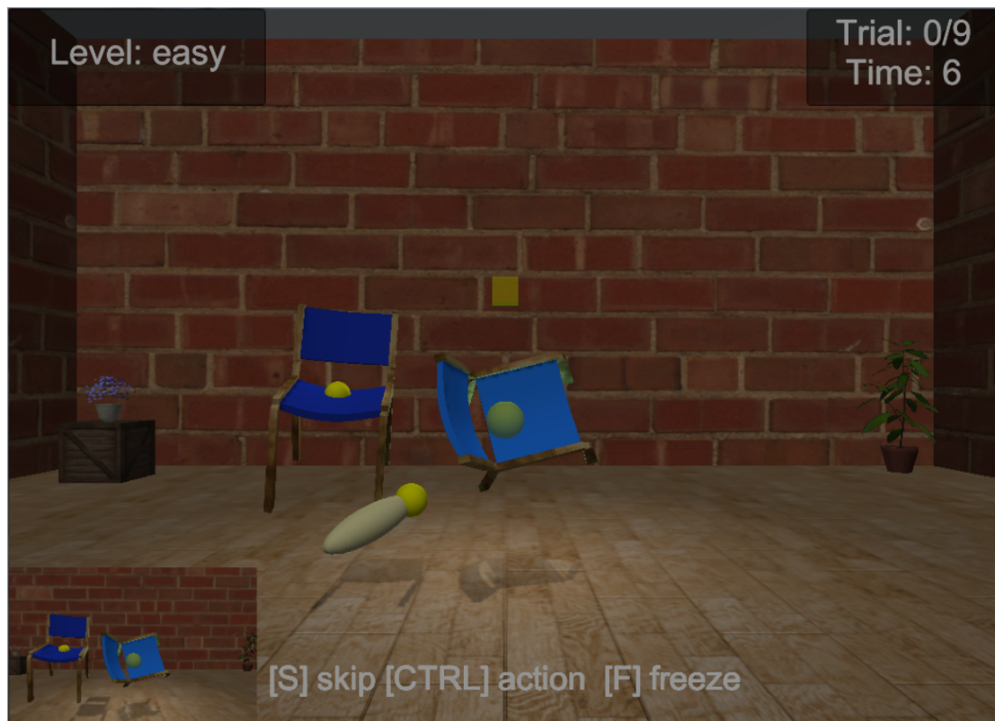
Fig. 4.1: The docking task environment. The virtual representation of the AirPen is visible in the image as an elongated ellipsoid. Bottom-left corner: the second camera offers six different views of the target. Top-right corner: the number of completed trials with the current input condition and the time elapsed since the trial began. Top-left corner: the difficulty level of the current task.
