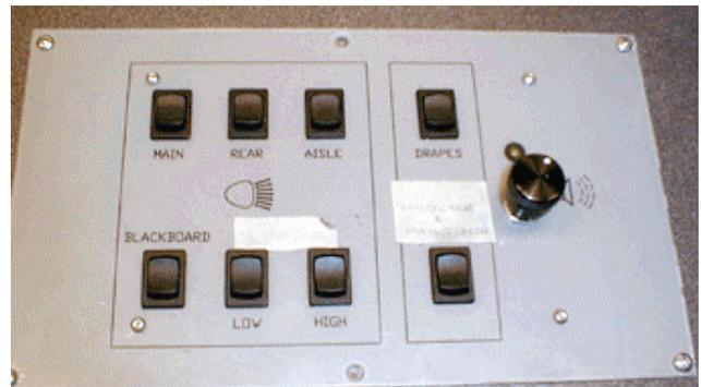
Figure 2. The HC-12 controlled physical button panel as an alternative to a graphical touch-screen interface. This panel provides manual override control of the room lights, projector, screen, drapes, and volume, without the need for distracting, hierarchical menus. Furthermore, the volume knob is context-sensitive, adjusting either the volume of the VCR when a tape is playing, otherwise, that of the instructor's microphone.
