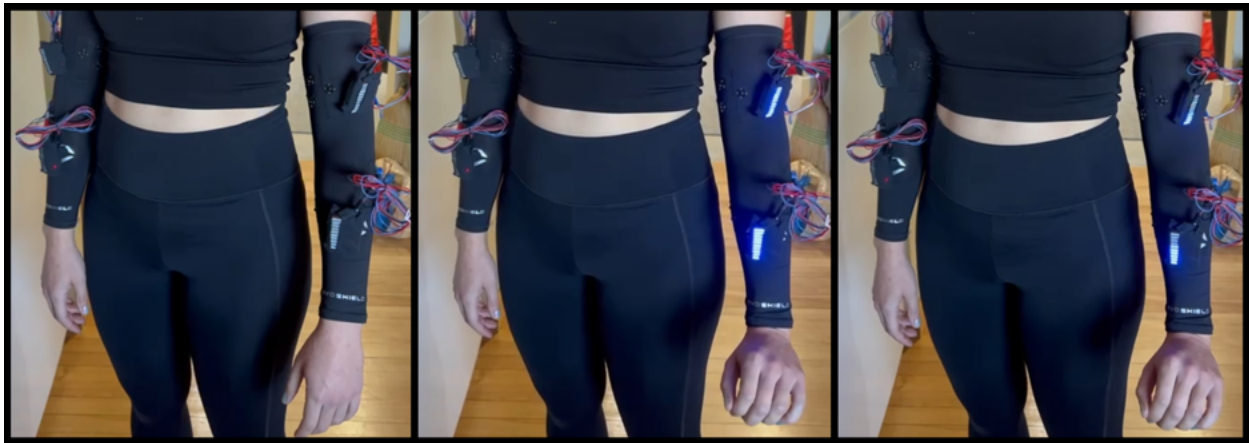
Figure 4.2: Demonstration of the MyoWare muscle sensors with LED displays. At rest (left), not enough muscle activation is detected to light up any LEDs. When flexing the wrist (middle), all ten LEDs light up, indicating significant muscle activity. After the initial activation (right), the muscle signal is not as strong, so fewer LEDs are on.
